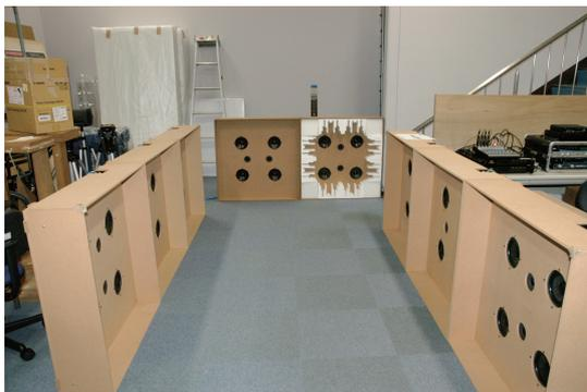
Fig. 1 photo of Variable Reflection Acoustic Wall System.
